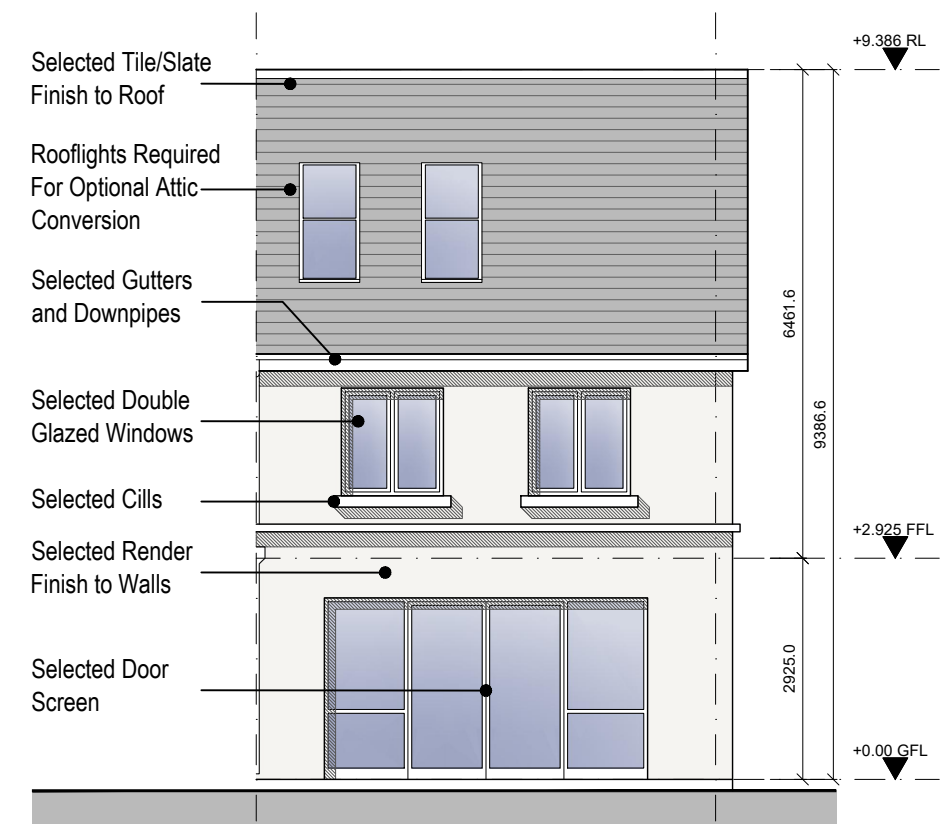
Type B1.1 Rear Elevation Scale 1:100
