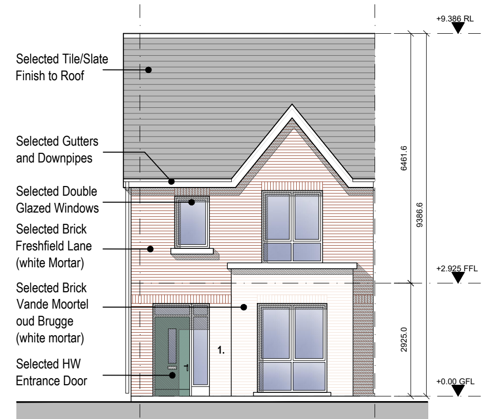
Type B1.1 Front Elevation Scale 1:100
